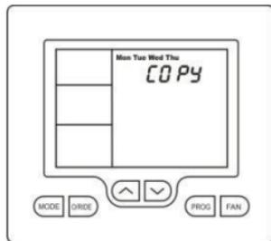
**Please Note** – Your thermostat’s programs may be controlled from a Building Management System (BMS) thereby overriding any program you may have entered, as described above. If the BMS is controlling the thermostat the word “Start” or “Stop” will flash in the LCD to indicate the thermostat program is under BMS control.
