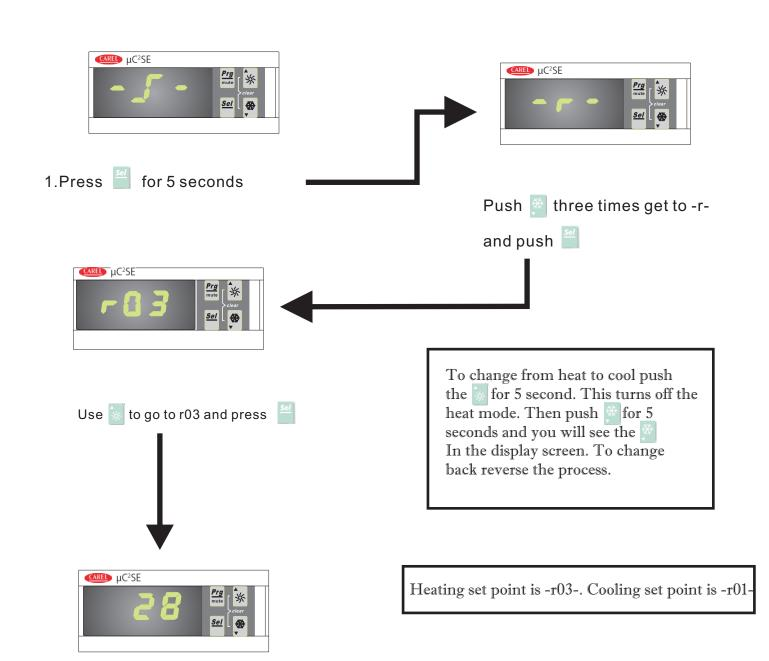
Use the or arrows to get to the desired setting and then push 3 times until you get back to the display temperature or leave for one minute and the display will go back to the display temperature
