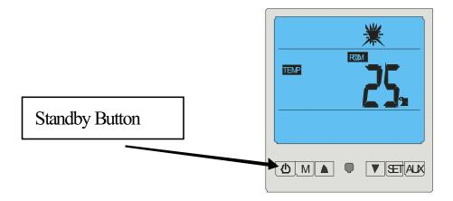
2. Press "SET" to find parameter 01 and then adjust up or down using arrows.
