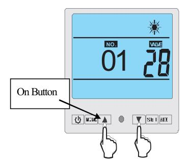
3. Wait 5 seconds and the ambient temperature will be displays. Then push the on button and the unit will turn on.
