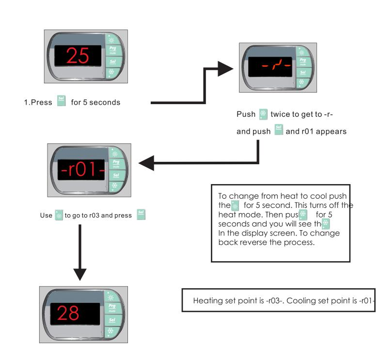
Use the or arrows to get to the desired setting and then push . This enters the setting. Push 3 times until you get back to the display temperature or leave for one minute and the display will go back to the display temperature
