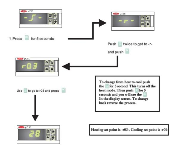
Use the or arrows to get to the desired setting and then push so 3 times until you get back to the display temperature or leave for one minute and the display will go back to the display temperature
